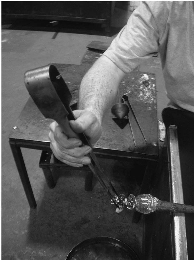
Figure 3.3 Instructor, Bill, jacking a caterpillar proficiently
