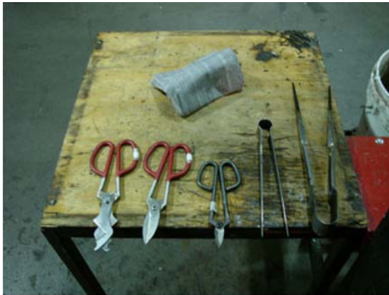
Tools on top of the workbench (right to left): jacks, tweezers, (extra set of specialized trim shears), shears, and diamond shears with folded wet newspaper behind.
